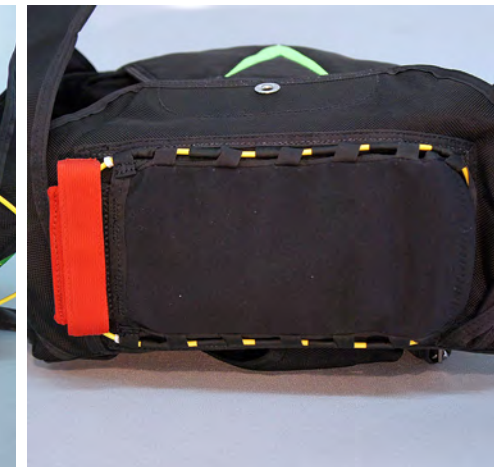
6. Thread yellow cable through loop under Type 12.
