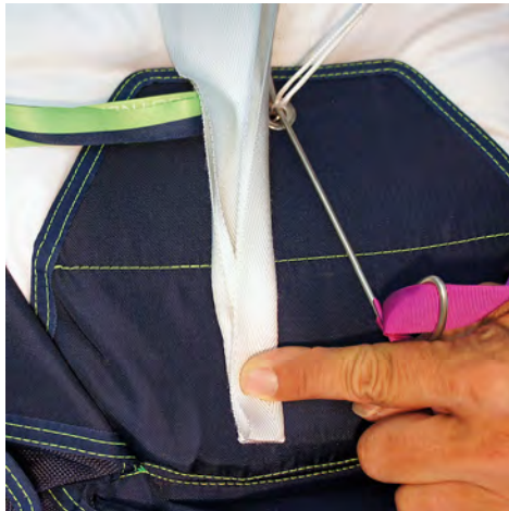
16. Tri-fold reserve bridle lengthwise.
