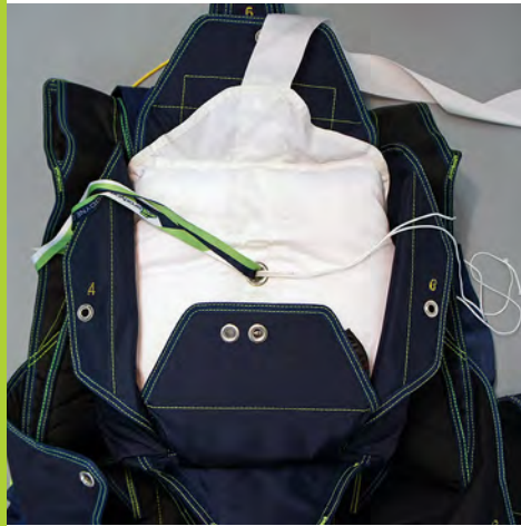
13. Rotate Freebag into reserve container filling lower corners of reserve container.
