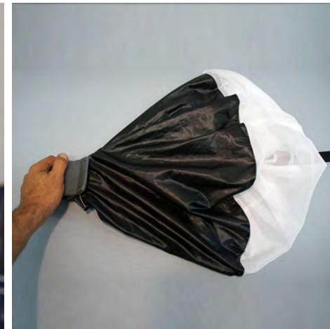
12. Pull the pilot chute to assure it is cocked.
