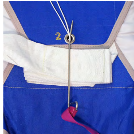
17. Close #2A cover flap and fold reserve crossways as shown.
