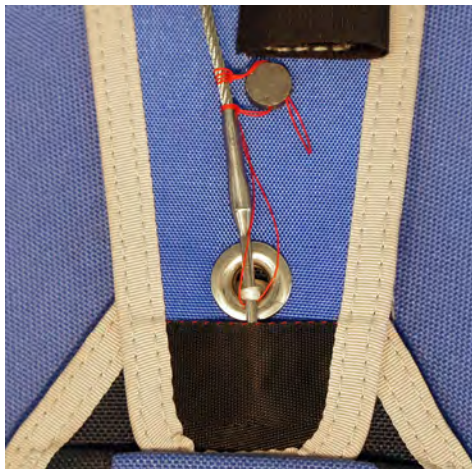
21. Seal with rigger's thread and lead seal per applicable regulations.
