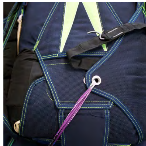
8. Pass the closing loop through the grommet on the right side flap (#3), making sure the bridle is exiting from the top right of the flap.
