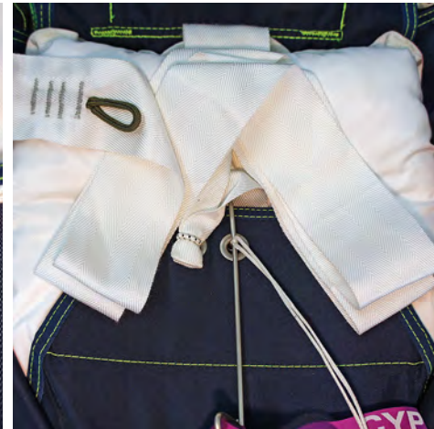
18. Fold bridle in "V" as shown.
