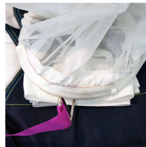
28. Ensure the lower spring coil is up against the spring ejector plate and that the excess bridle sits under the pilot chute without catching the fabric under the spring.
