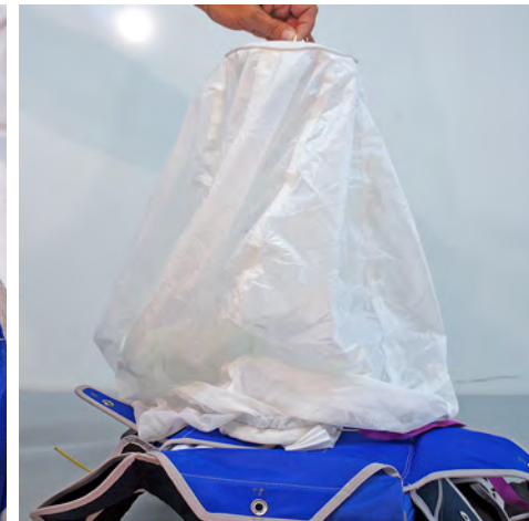
18. Pass the pull up cord cleanly through the pilot chute from bottom to top plate.
