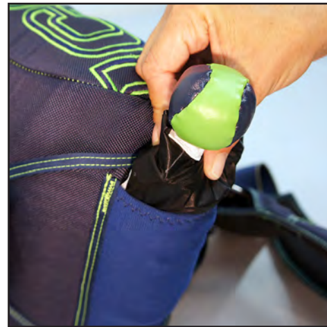
9. Stow pilot chute in BOC Pocket as shown.
