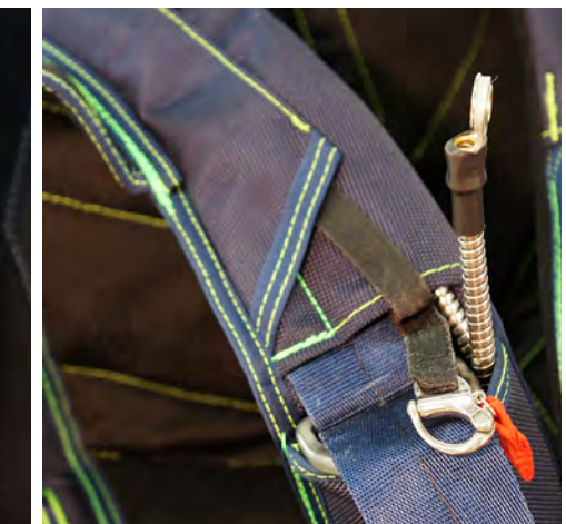
4. RSL Prepared and ready for connection to Riser.
