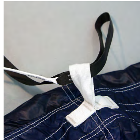
8. Thread the end loop of the bridle through the canopy's attachment point.
