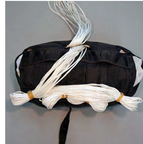
10. D-Bag ready to be placed in Container.
