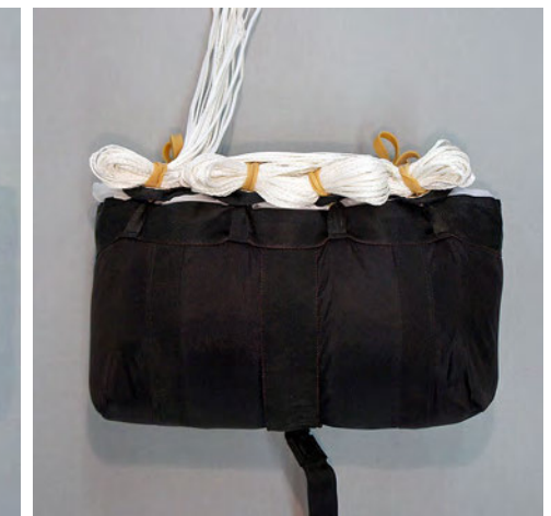
3. Stow the second center stow as shown. Continue stowing the top stows, starting at the mouth of the D-Bag.
