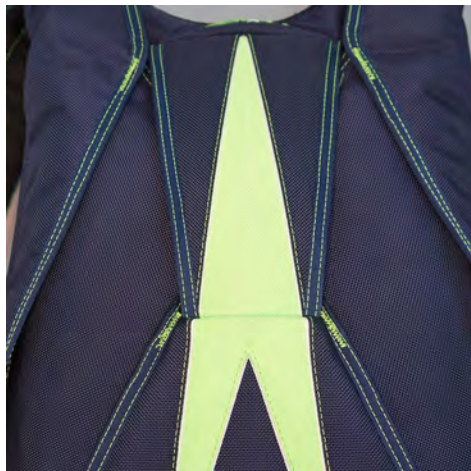
38. Close the final cover flap and tuck the tabs under the #6 flap.
