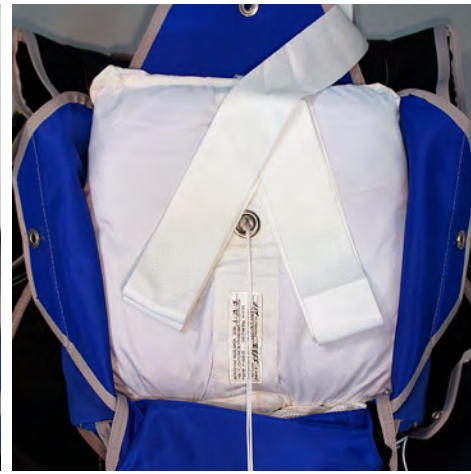
14. Fold the reserve pilot chute in a V-shape pattern as shown. Leave a minimum of 4 ft of reserve to base of reserve pilot chute.
