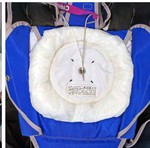
21. Neatly roll the Pilot Chute Fabric up against the outer rim of the Reserve Pilot Chute. Do not tuck the Reserve Pilot Chute Fabric under the lateral closing Flaps #3 and #4.
