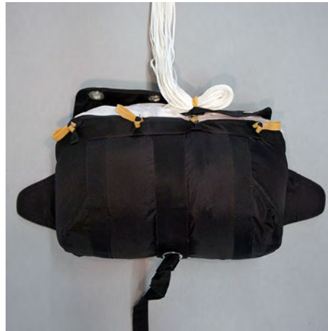
2. Stow the first center stow as shown.
