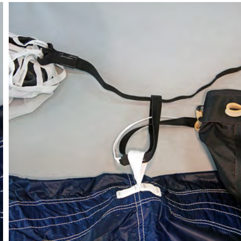
9. Thread the pilot chute and D-bag through the bridle's end loop.
