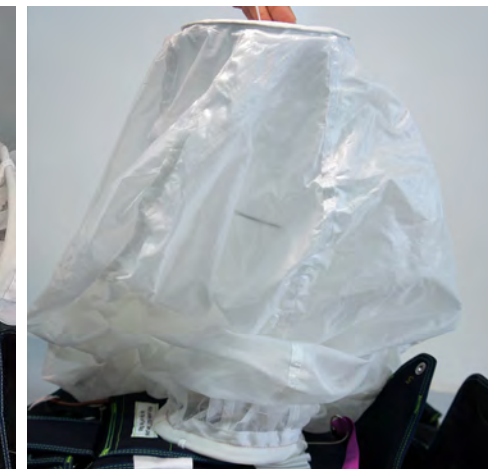
27. Pass the pull up cord cleanly through the pilot chute from bottom to top plate.
