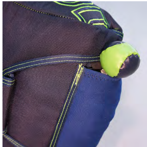
10. Ensure pilot chute is secure and can be accessed by jumper.
