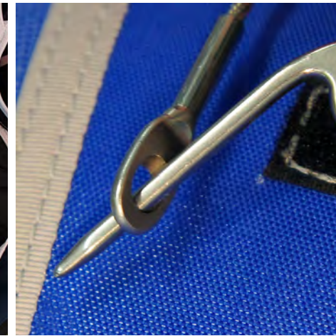
26. Insert the reserve pin through the eye of the reserve cable. Make sure pin is inserted in the same direction as the angle of the opening in the ripcord's eye.
