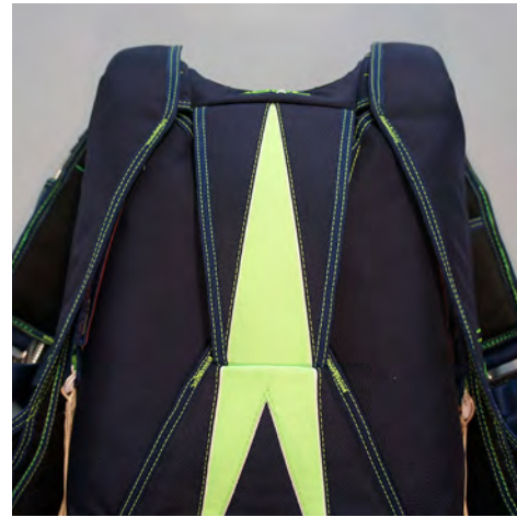
2. Close riser covers over the risers
