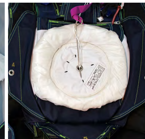
30. Neatly roll the Pilot Chute Fabric up against the outer rim of the Reserve Pilot Chute. Do not tuck the Reserve Pilot Chute Fabric under the lateral closing Flaps #3 and #4.
